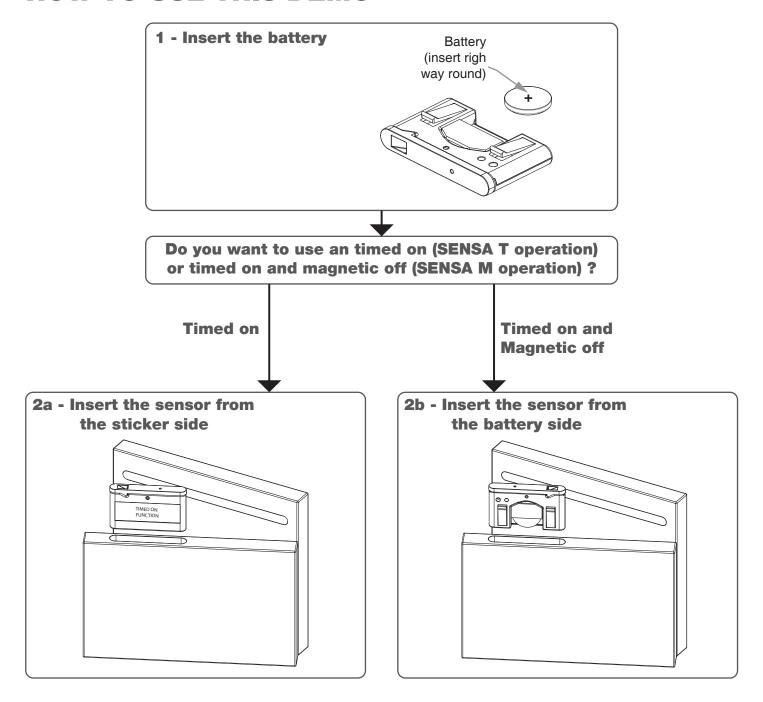
NOTE: The sensor is already associated in the control unit. When you insert the battery it immediately starts to work.
